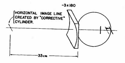
In the figure above, the  $-3 \times 180$  corrective lens moves the horizontal line which was 3 D in the vitreous back onto the retina.
