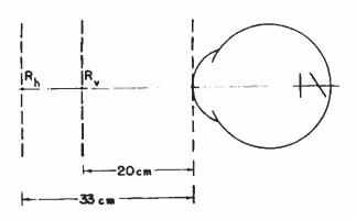
To "correct" this eye, we have to go through the same procedures as for the spherical refractive error — we have to place the corrective lens so as to image infinity at the far point; (the lens can be located at whatever position you choose if its power is appropriately adjusted). However, for the astigmatic eye there are two far points, so this procedure must be done for both primary meridians using a cylindrical lens for each.
