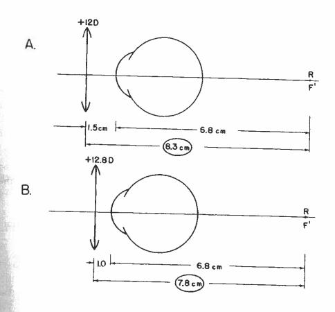
But he is wearing a + 12.0 D lens inadvertently fitted at this 10 mm vertex distance, so he is *under*corrected in plus power by (12.8 - 12.0) or 0.8 D — certainly not an *in*significant amount.
