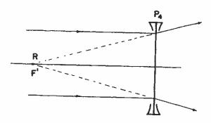
If the corrected lens were located at position 3 above, it would of necessity have a shorter secondary focal length and, therefore,  $P_3$  would be greater in minus power than  $P_4$ . Of all the possible corrective lenses, the one with the *least* minus power would be situated furthest away from R, that is, in contact with the corneal surface — a contact lens of — 7 D power.
