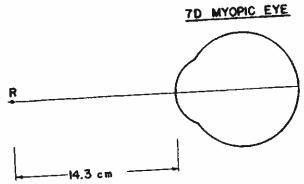
A "corrective" lens is placed so as to take parallel light bundles from infinity and, after refraction by the lens, make them seem to the eye as if they arose at R. Such a lens will do so only if its secondary focal point F' coincides with R.
