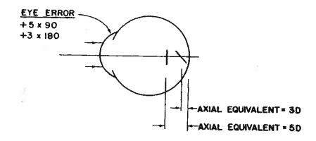
Since the horizontal line-images of each object point are positioned closer to the retina, the horizontal lines making up any target or test letter located at infinity will appear clearer than will the vertical strokes. For this eye, a target letter H would look something like that shown below — each object point being represented on the retina as a horizontal ellipse.
