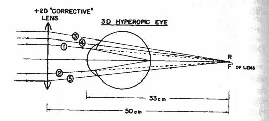
In the figure above, rays 3, 4 and 5 are blocked by the sclera and do not get through the pupil; therefore, they cannot help form the retinal image point. In this figure, only those rays between 1 and 2, imaged by the lens at R, actually enter the eye and are imaged by it sharply on the retina. 1 and 2 are "limiting" rays — limited by the edge of "the pupil".
