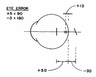
The + 5  $\times$  90 means the vertical line is 5 D in front of the retina; the - 3  $\times$  180 signifies the horizontal line image is 3 D "behind" the retina. These lines are separated by 8 D, that is, the astigmatic error
