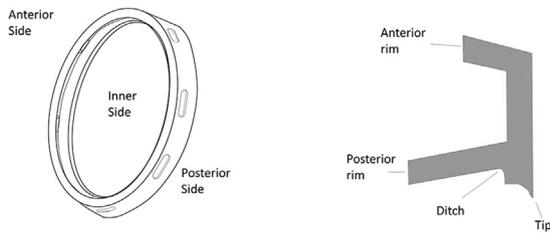
**Figure 4.** Illustration of the open-capsule device. *Left:* Overview. *Right:* Side view. The presence of the anterior rim or “roof” keeps the capsule away from the anterior IOL surface. Drawings modified from Alon et al.<sup>26</sup>
