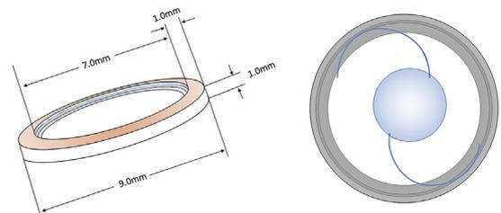
**Figure 1.** The endocapsular equator ring. *Left:* Overview. *Right:* Anterior view with a standard IOL positioned within the ring. Drawings modified from Hara et al.<sup>13</sup>
