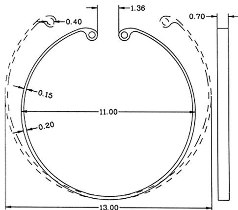
**Figure 2.** The capsular bending ring with associated dimensions. Reprinted with permission of the *Journal of Cataract & Refractive Surgery*.<sup>24</sup>
