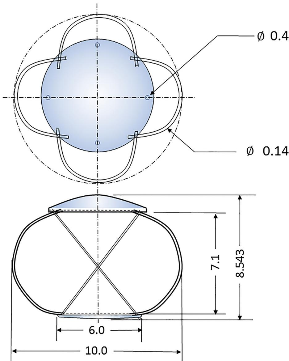
**Figure 7.** Schematic drawings of the spring-loaded IOL. *Top:* Anterior view. *Bottom:* Side view. Drawings modified from Hara et al.<sup>31</sup>
