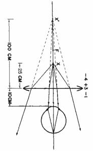
That is, although the actual rays (shown in solid lines) are divergent as they leave lens P, they simulate rays (dotted lines) which would have come from a real point located 100 cm away. All real, honest-to-goodness light rays will, in the diagrams of this book, be indicated as solid lines, while rays from apparent (virtual) points will be shown as dotted lines).
