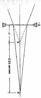
Let u — the distance from our lens to the image at X (which would have been produced by the projector if the lens did not intercept the rays first!) This is the object distance for our — 2 D lens. The object vergence  $U = +\frac{1}{u}$ : P = -2; the image vergence  $V = +\frac{1}{(.25 + u)}$ .
