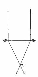
the two rays drawn, of course, signify light emanating from one point (the axial one) of a very distant object as they are brought to a point focus at F'.
