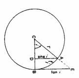
We have drawn the circle above with its center at C and two radii, CA and CB, and constructed two perpendicular lines to radius CB; one is dropped from the end of radius CA, the other at the end of radius CB.
