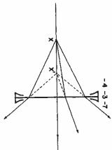
This locates an image point at  $-\frac{1}{7D}$  or -14.1 cm, the minus sign again meaning "to the left of lens P".
