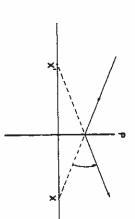
away from the axis, divergence must have been added by it; therefore the lens to that single light ray. Since the light ray is bent upwards. were directed from axial point X'. Again note only what happens at be virtual). After a ray drawn toward X hits lens P, it will act as if it convergent (at the lens plane) toward object point X (which must thus The only difference with X on the right is that this signifies that light is P here must be a minus lens. In this example both X and X' are virtual
