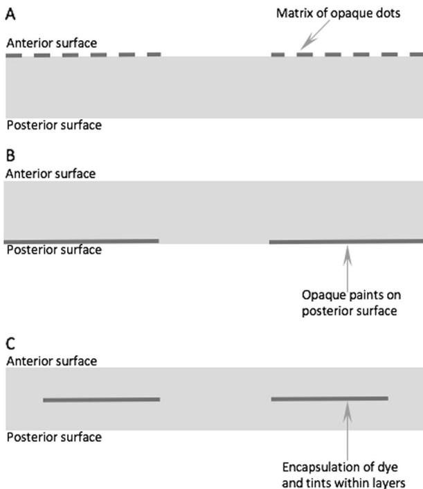
**Fig. 3** An illustration of dot-matrix (a), opaque backing (b) or laminate construction (c) techniques to apply opaque tints to cosmetic contact lenses
